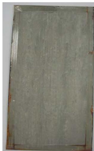
(b) 80/20 Sn/Zn passivado com  $\text{Cr}^{3+}$  (3  $\mu\text{m}$ )
