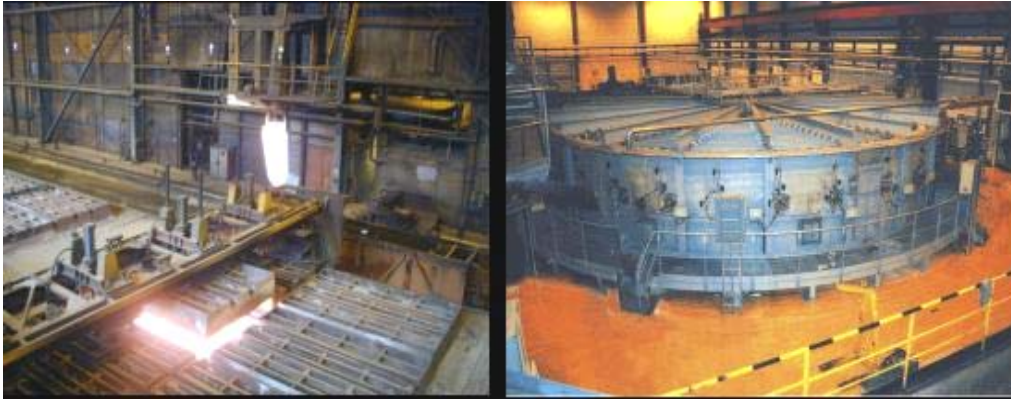
Figure 1. Ovako, Hofors works, Sweden, has since 1994 implemented oxyfuel in 48 pit and 2 rotary-hearth furnaces for greater throughput capacity, providing flexibility fuel savings and reduced emissions.
