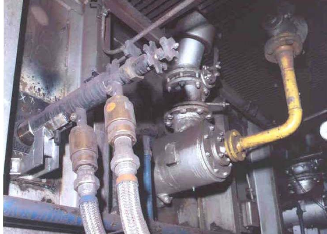
Figure 6 Oxyfuel burners are both compact and powerful. In this boosting application an additional 2 MW oxyfuel burner (left) are placed next to an existing 0.5 MW airfuel burner (right).
