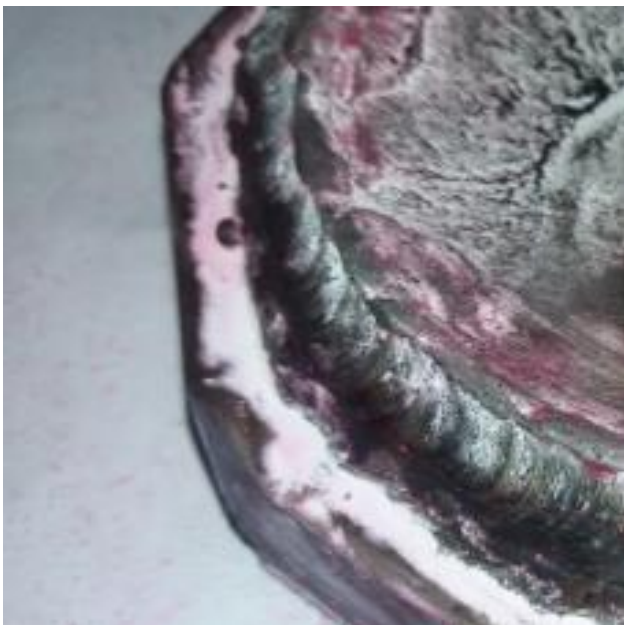
Figure 12. Welding as a tension concentrator
