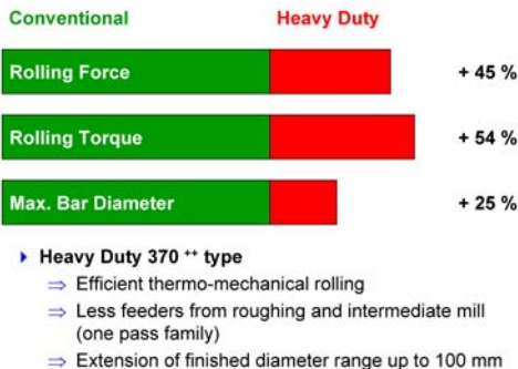
Figure 4: Comparison of basic data of conventional and heavy duty 370 ++ stand
