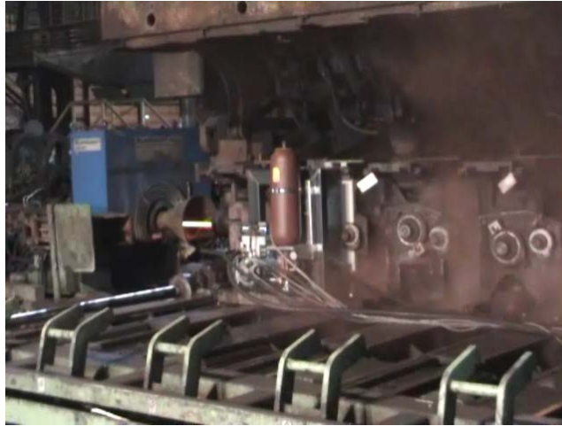
Figure 10: View of the new Stand A Adjustable U nder L oad (AUL) in operation
