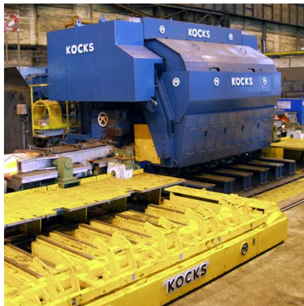
Figure 1: First 3-roll heavy duty R educing & S izing B lock operating at Saarstahl AG
