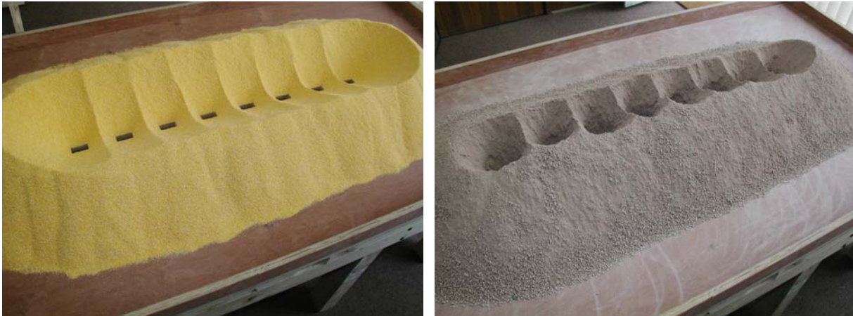
Figure 3. Scale model of a prismatic stockpile handling different materials.
