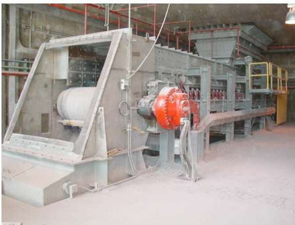
Figure 4. Belt feeder and details of a mass flow interface.
