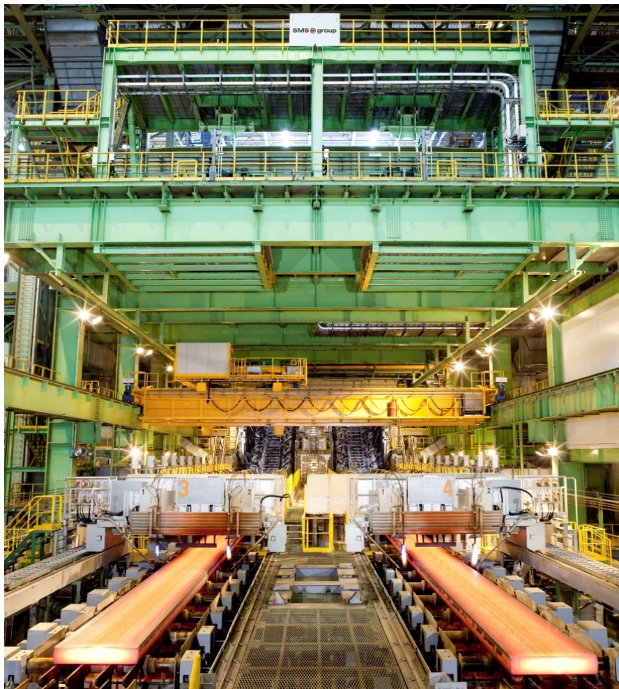
Figure 1. With HD scan the quality of the slabs is checked quickly and easily.
