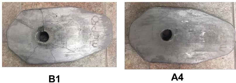
Figure 11. External appearances of SV plates after commercial applications at steel mill B.
