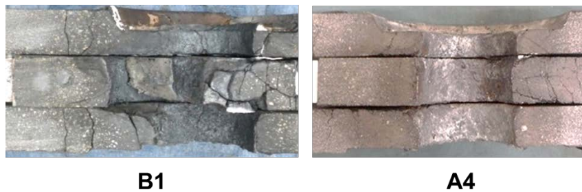
Figure 12. Cut surfaces of SV plates after commercial applications at steel mill C.
