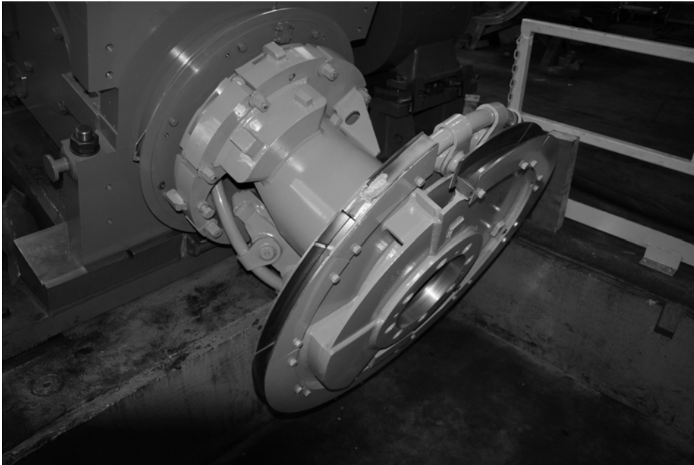
Figure 11 – Laying Head Tail End Control Arrangement
