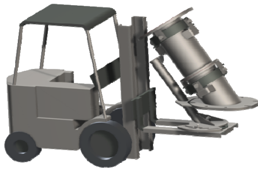
Handling and dismantling device for downleg
