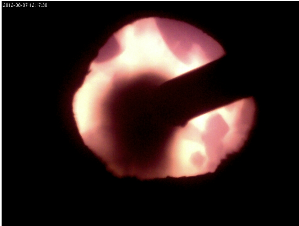
Figure 2. Sample showing pulverized coal injection.
