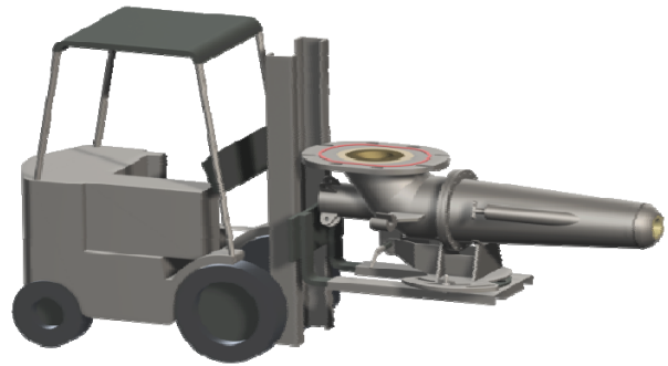
Handling and dismantling device for elbow and blowpipe
