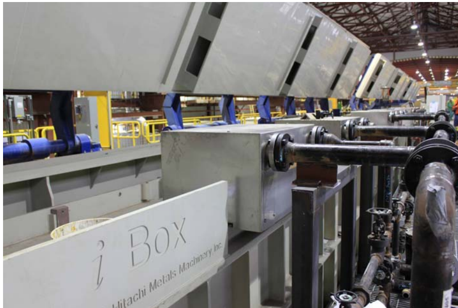
Figure 8. Overview of i Box pickling tank made of Polypropylene (PP).
