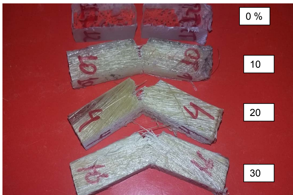
Figure 2 - Macrophotograph of Izod impact tested specimens with different amounts of continuous and aligned palm fabric - epoxy composites
