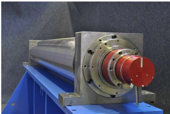
Figure 2: Latest generation X-Shape flatness measuring roll as developed by SMS Siemag (l). Design of the rotary transmitter and signal processing (r)
