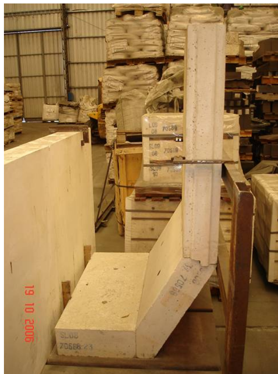
Figure 9: Pre cast security lining
