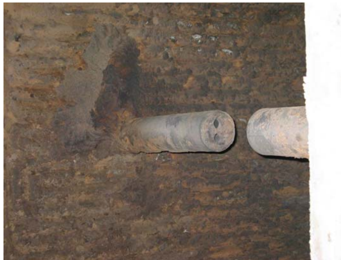
Figure 6. The lances after three month of operation.
