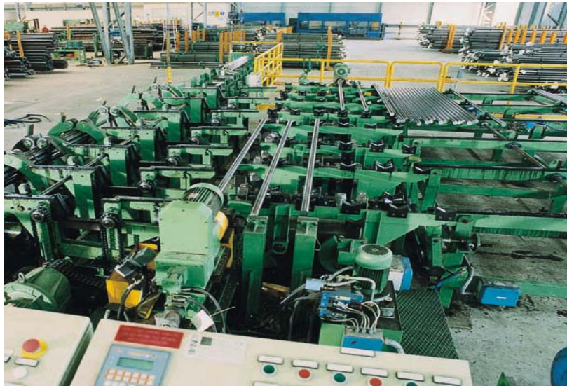
Figure 4. Bar chamfering station.
