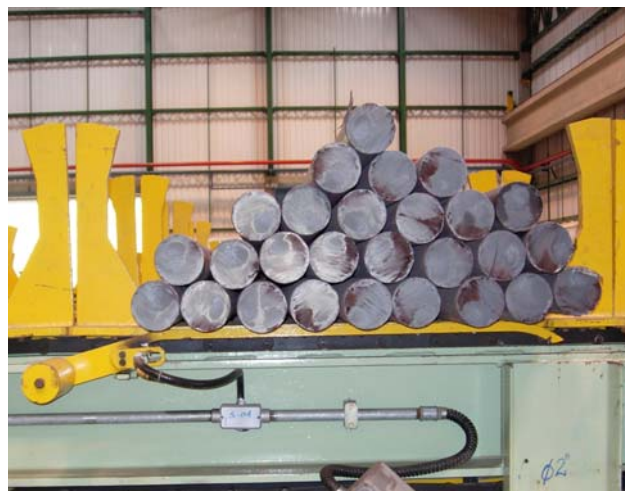
Figure 1. Bar loading transfer for 3 bundles.
