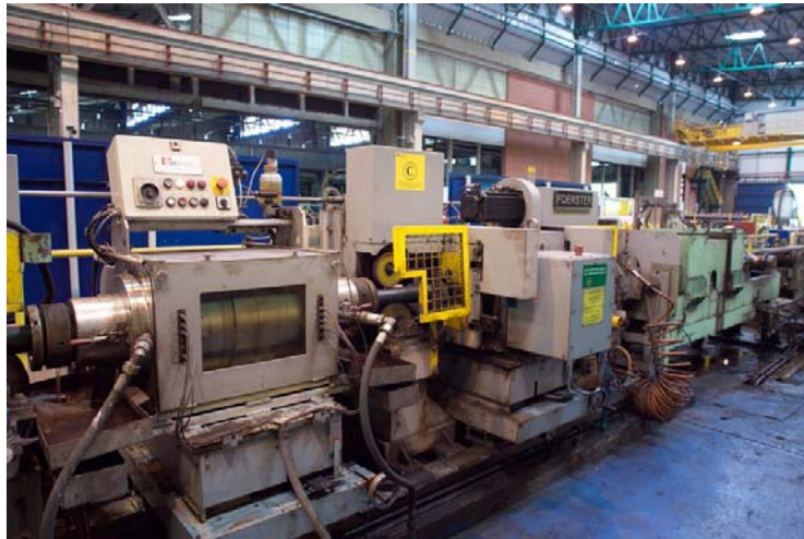
Figure 5. Ultrasound and flux leakage non destructive testing station.
