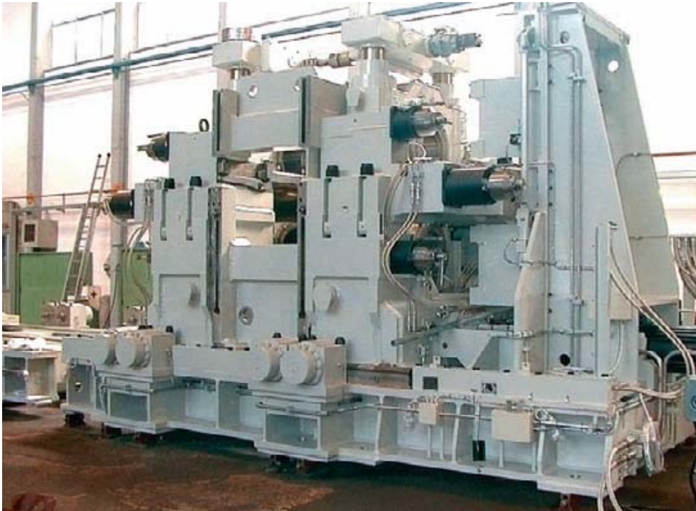
Figure 4. Universal stand on baseplate with spindle holder.
