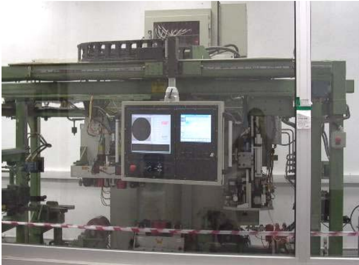
Figure 11. Eddy-current testing unit.
