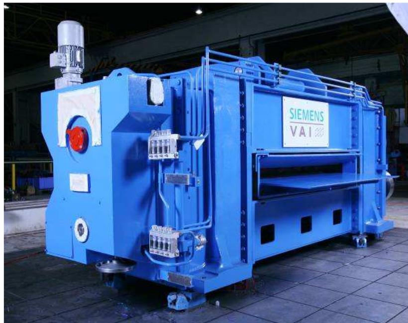
Figure 5: Rotary Shear in Siemens VAI MT workshop in
