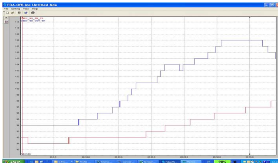
Figure 10 – trends of outlet and inlet temperatures in water cooled panels in the Jacksonville EAF.
