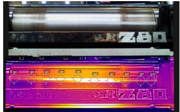
Figure 5: Real and thermographic image of rolls table.
