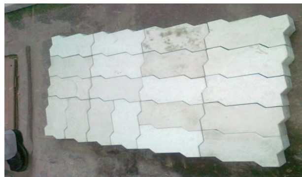
Figure 6 Paving blocks from synergistic use of granulated blast furnace slag and fly ash
