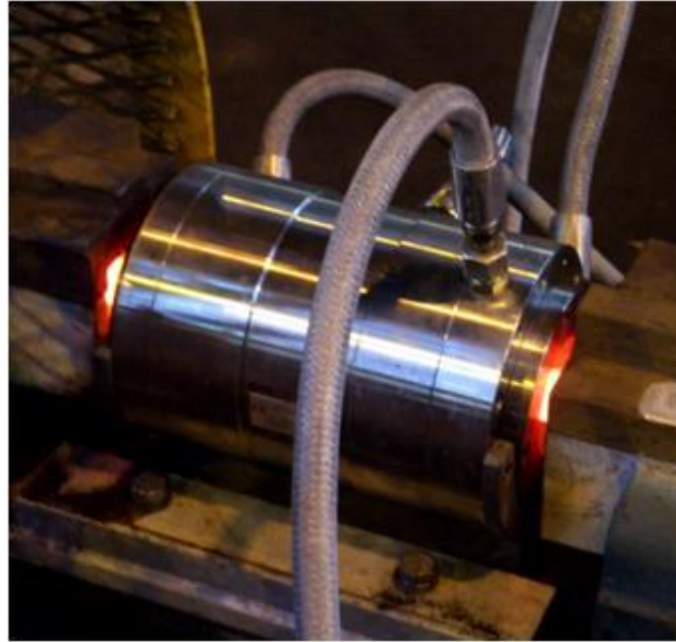
Figure 1. HiSECTION - non-contact eddy current system for in-line measurement of cross sectional area of hot-rolled bars.
