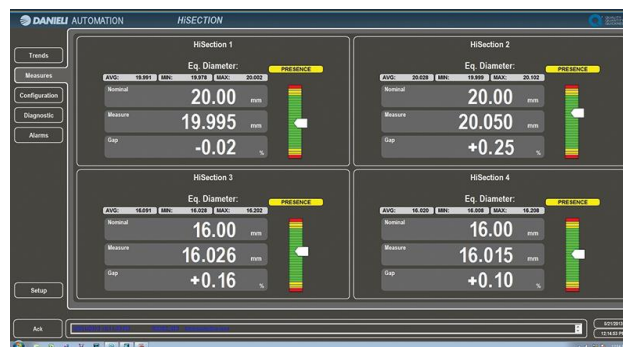
Figure 2. HiSECTION - HMI workstation interface.
