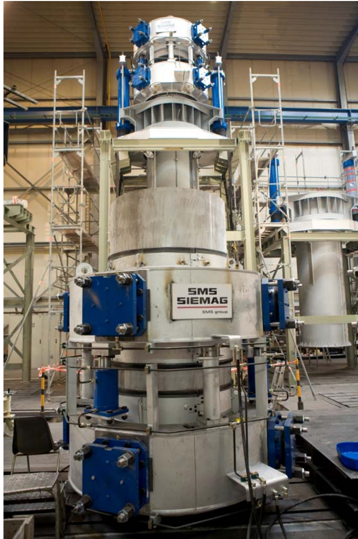
Figure 2. Electrode slipping device of a submerged-arc furnace.
