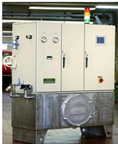
Figure 2: Tank, pump and control unit of the low quantity lubrication
