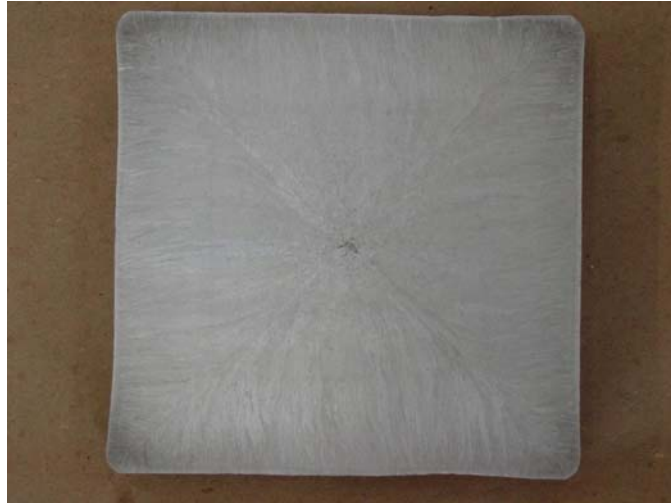
Figure 6. Macro etch of 304 Stainless steel, casting speed 1.6 m/min.
