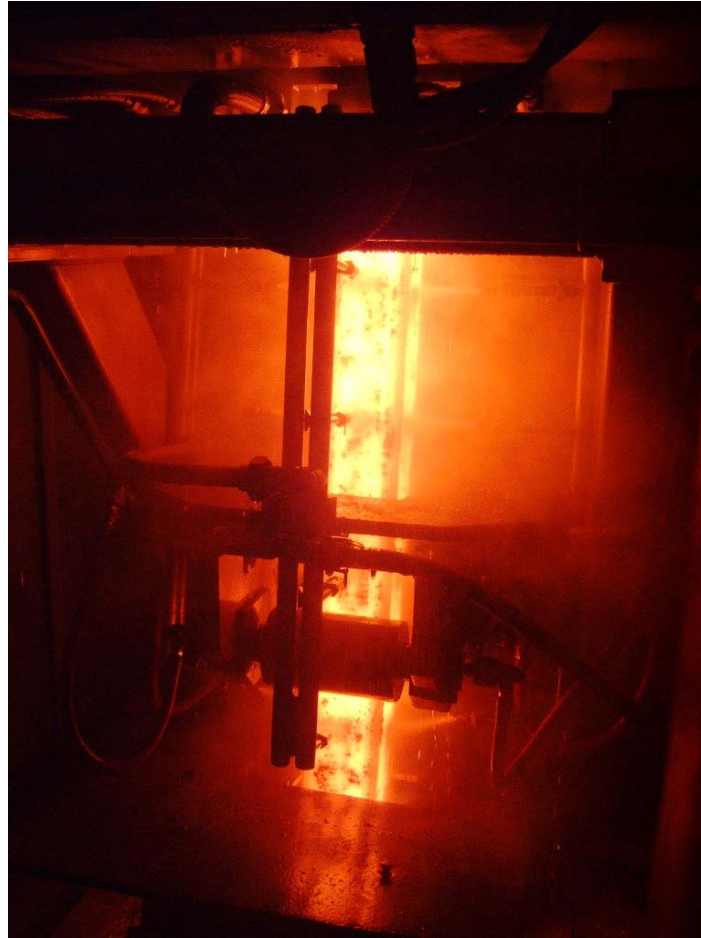
Figure 5. Secondary cooling area.
