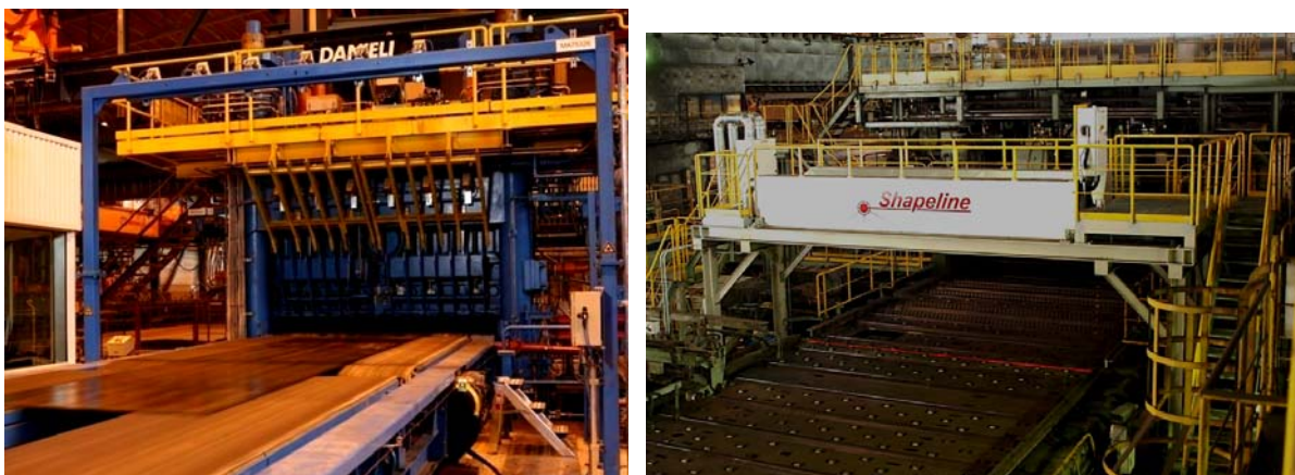
Figure 8. Left: The lasers have been integrated onto the leveler (behind the steel bars) and the cameras far away (on the blue structure in the front) to allow for extreme skew of the plates. Still the point of measurement can be chosen to be on an optimal distance from the leveler. From SSAB, Oxelösund, Sweden. Right: The lasers, cameras, cooling system and electronics are integrated on a common platform, protected by heat-shields underneath and accessible through stairs from both sides of the line. All components are accessible and replaceable also when the line is running. At the measurement position (where the laser lines are), the plate is supported by non-driven support rolls to eliminate elastic deformation of the plates. From Nippon Steel, Oita, Japan.
