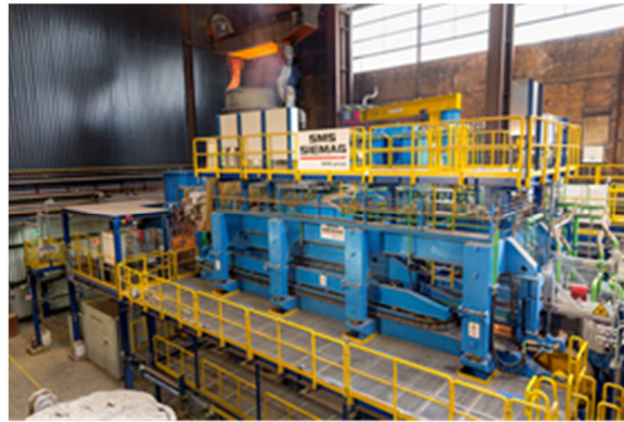
Figure 2. Set-up of BCT® caster in Peine.
