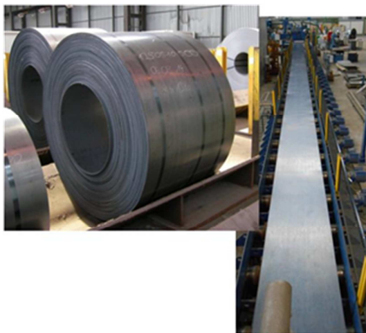
Figure 6. Hot rolled carbon steel strip (2.5mm) after laminar cooling on the exit roller table of the rolling mill (right); Hot strip coils build up by plasma welding of several strip pieces (left).
