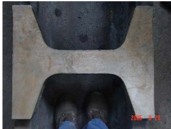
Figure 9: Macro etch sample of a near-net-shape beam blank.
