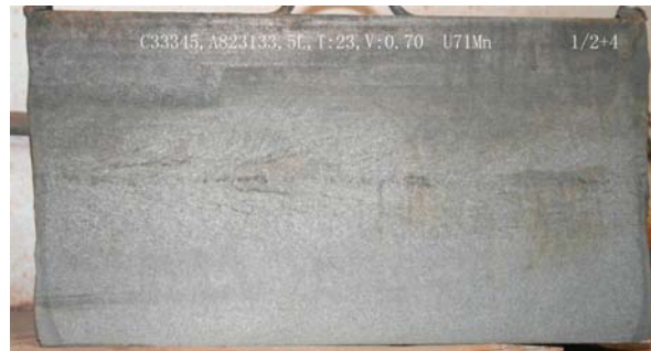
Figure 6: 280x380 mm Rail bloom with dynamic soft reduction.
