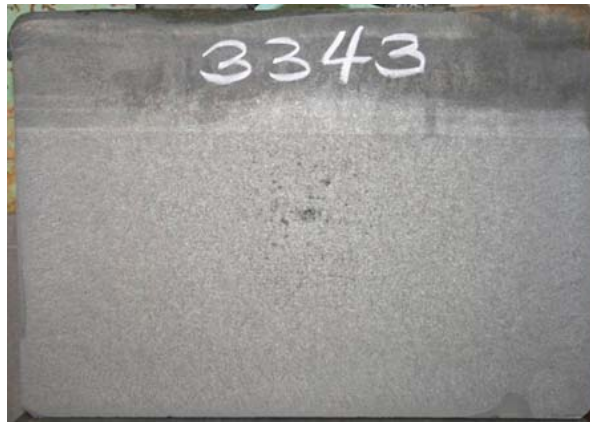
Figure 5: 280x380 mm Rail bloom with dynamic soft reduction.
