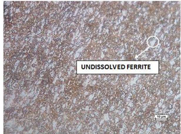
Figure 3. Optical Micrograph of sample subjected to Intercritical heat treatment at 800°C – Etched with 3% Nital original magnification 500x.
