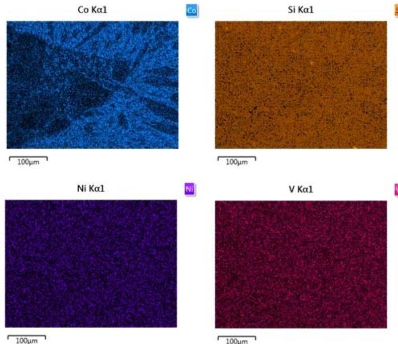
**Figure 8.** EDS mapping results in between the "rice crispy" and the CCO matrix for Cobalt, Silicon, Nickel and Vanadium
