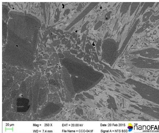
**Figure 6.** Backscattered SEM showing the area of the "rice crispy" selected for EDS analysis
