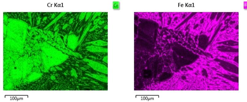
**Figure 7.** EDS mapping results in between the "rice crispy" and the CCO matrix for Iron and Chromium
