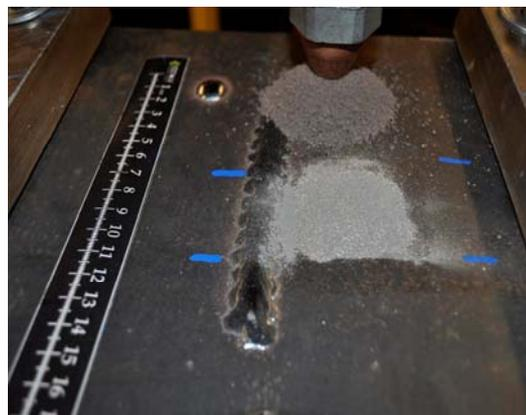
**Figure 1.** Addition of alloying elements on CCO 's submerged arc welding
