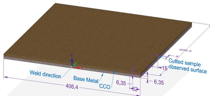
**Figure 2.** Sketch showing CCO plate, location and dimensions of the sample
