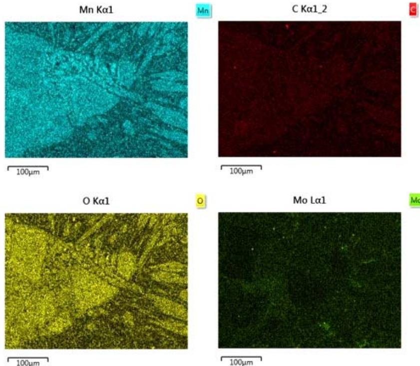
**Figure 9.** EDS mapping results in between the "rice crispy" and the CCO matrix for Manganese, Carbon, Oxygen and Molybdenum
