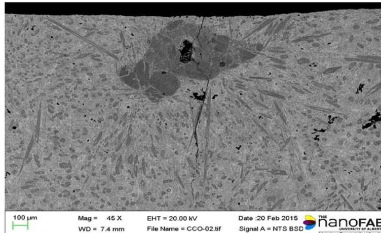
**Figure 5.** Backscattered SEM showing the "rice crispy" with a porosity in the center and a crack passing through.
