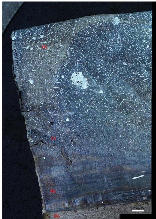
**Figure 4.** Mosaic microstructure 50X, etchant 20 ml H<sub>2</sub>O, 10 ml HCl, 30ml HNO<sub>3</sub> and 5 g FeCl<sub>3</sub>. A) Base metal B) Mixed zone C) Intermediate Zone D) CCO Top zone.
