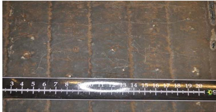
**Figure 3.** Surface top view of industrial SAW CCO sample showing cracks and bead overlap recess
