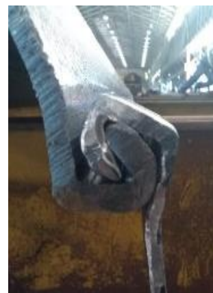
Figure 18. Lock formation in the first hot test
