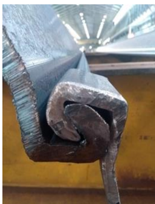
Figure 20. Lock formation in the last hot test
