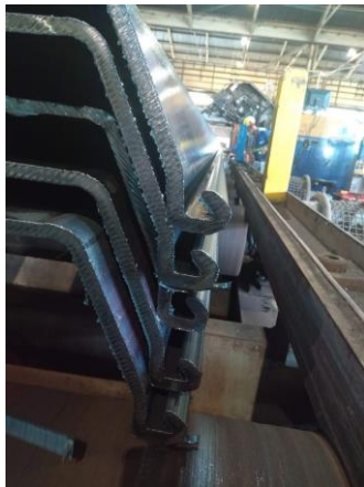
Figure 25. Lock formation after last pass – hot mill trial
