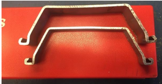
Figure 24. Lock formation after last pass – Lab Mill
