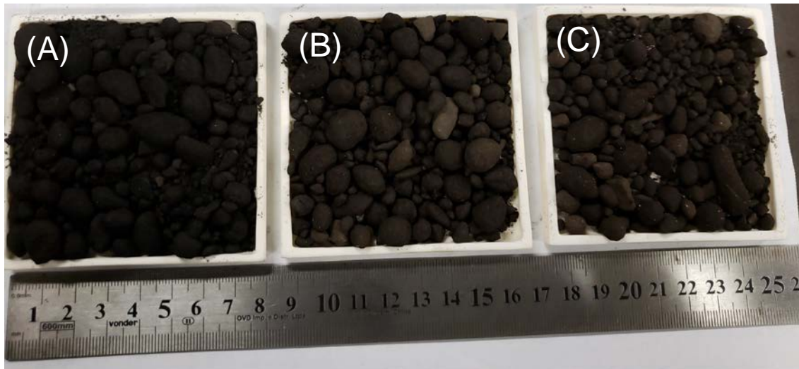
Figura 3. Quase-partículas mistura (A) coating fino, (B) coating grosso e (C) sem coque.
