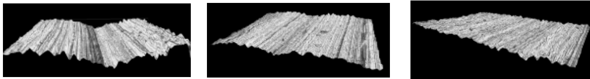
a) 0.6 mm rev -1 b) 0.3 mm rev -1 c) 0.15 mm rev -1 Figure 6. Digital surface reconstruction for a constant cutting speed of 120m min -1
