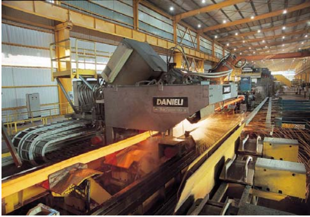
Figure 1. EWR® Billet Welding Line in operation.
