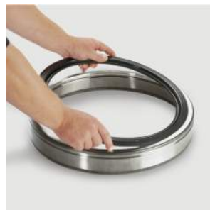
Figure 8 - Disassembly of bearing cage.
