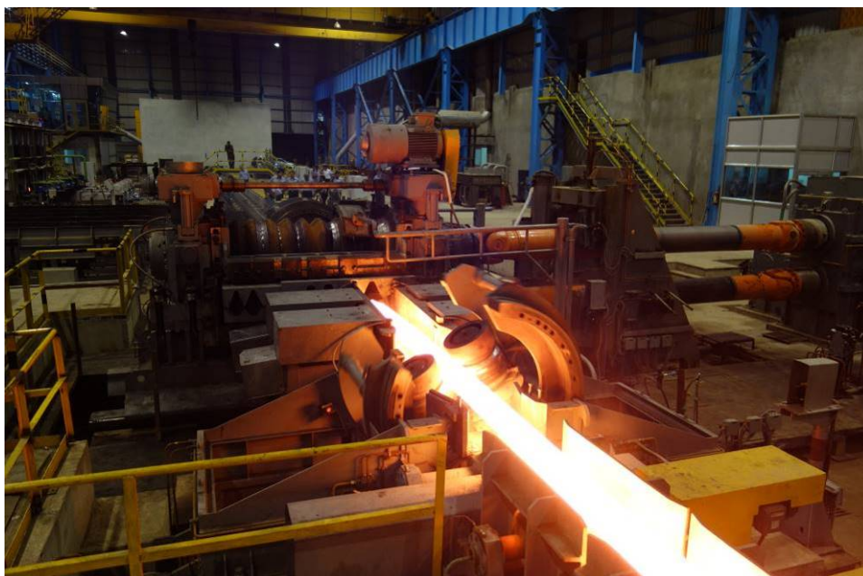
Figure 2 – Reversing sliding breakdown with bar rotating device
