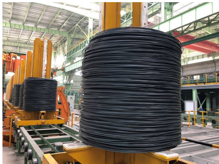
Figure 12 – Vertical pallet coil handling system
