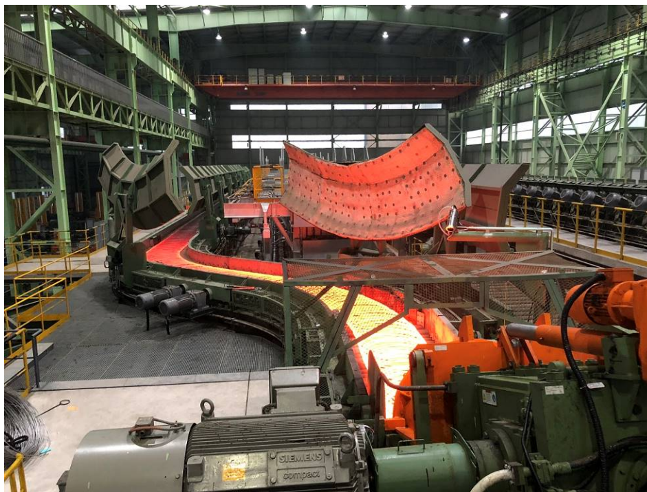
Figure 9 - Stelmor and DST Lines
