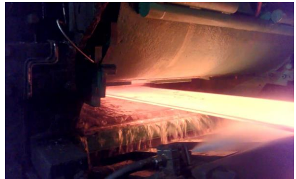
Figure 4. Strip surface at FM2 exit.
