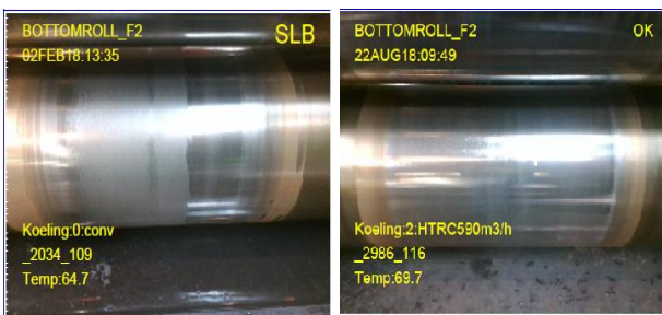
Figure 8. Examples of banding (left) and no banding (right) of the roll surface.
