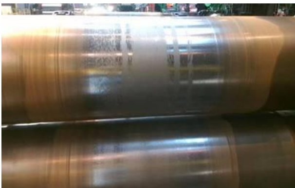
Figure 14. Poor roll surface quality (banding) after rolling a 1.8 mm heavy HSLA grade.
