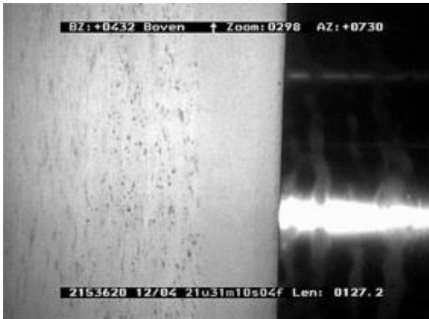
Figure 7. Typical salt and pepper scale defect.
