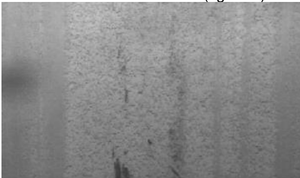
Figure 8. Typical peeled roll scale defect.
