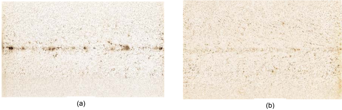
Figure 7. Comparison of internal quality of C45 billet of section 350 × 320 mm (a) without DSR; and (b) with DSR.
