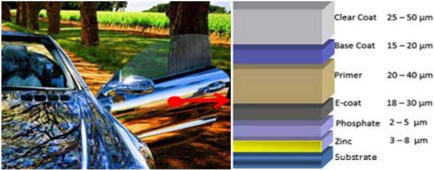
Figure 1: The layers: from substrate to clear coat. (8)
