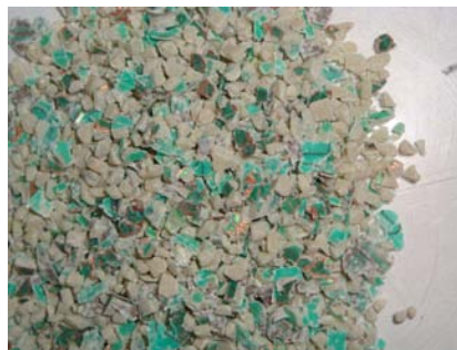
Figure 2. Particles \leq 3.0 mm nude printed circuit board after knife mill.
