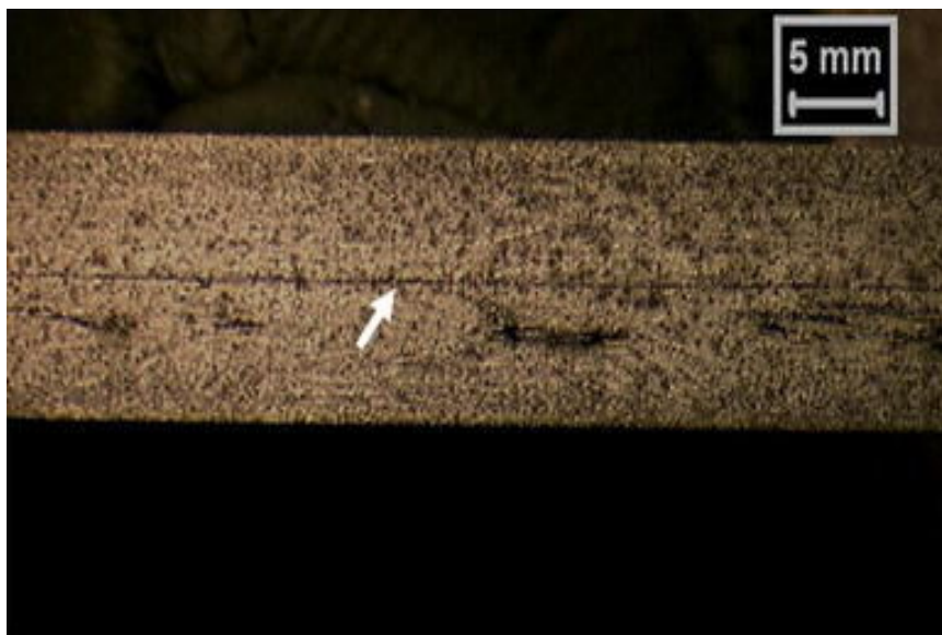
Figure 1. Crack-like defect at slab or billet centerline [2]
