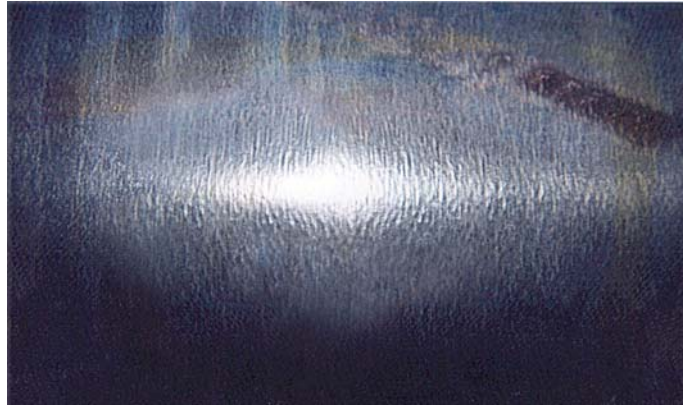
Figure 6: Hot-work tool steel roll in a European rolling mill after 150,000 t.
