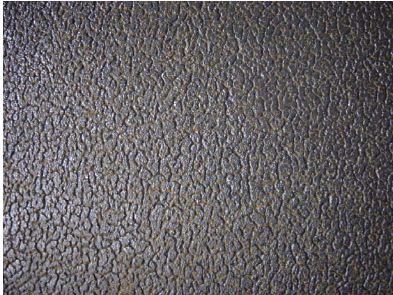
Figure 5: High-chrome steel roll after 3 weeks of use in a two-high stand.
