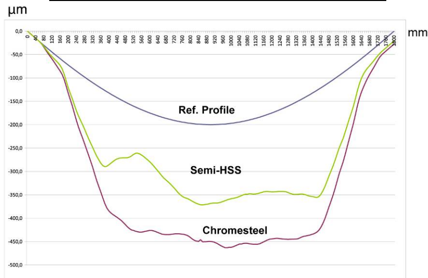
Figure 2: Wear profile for top rolls after approx. 25,000 t.
