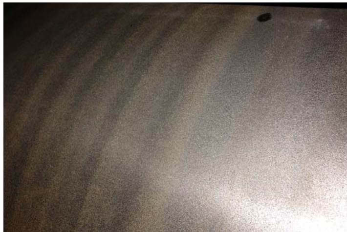
Figure 7: Hot-work tool steel roll in an Asian continuous stand after 300,000 t.
