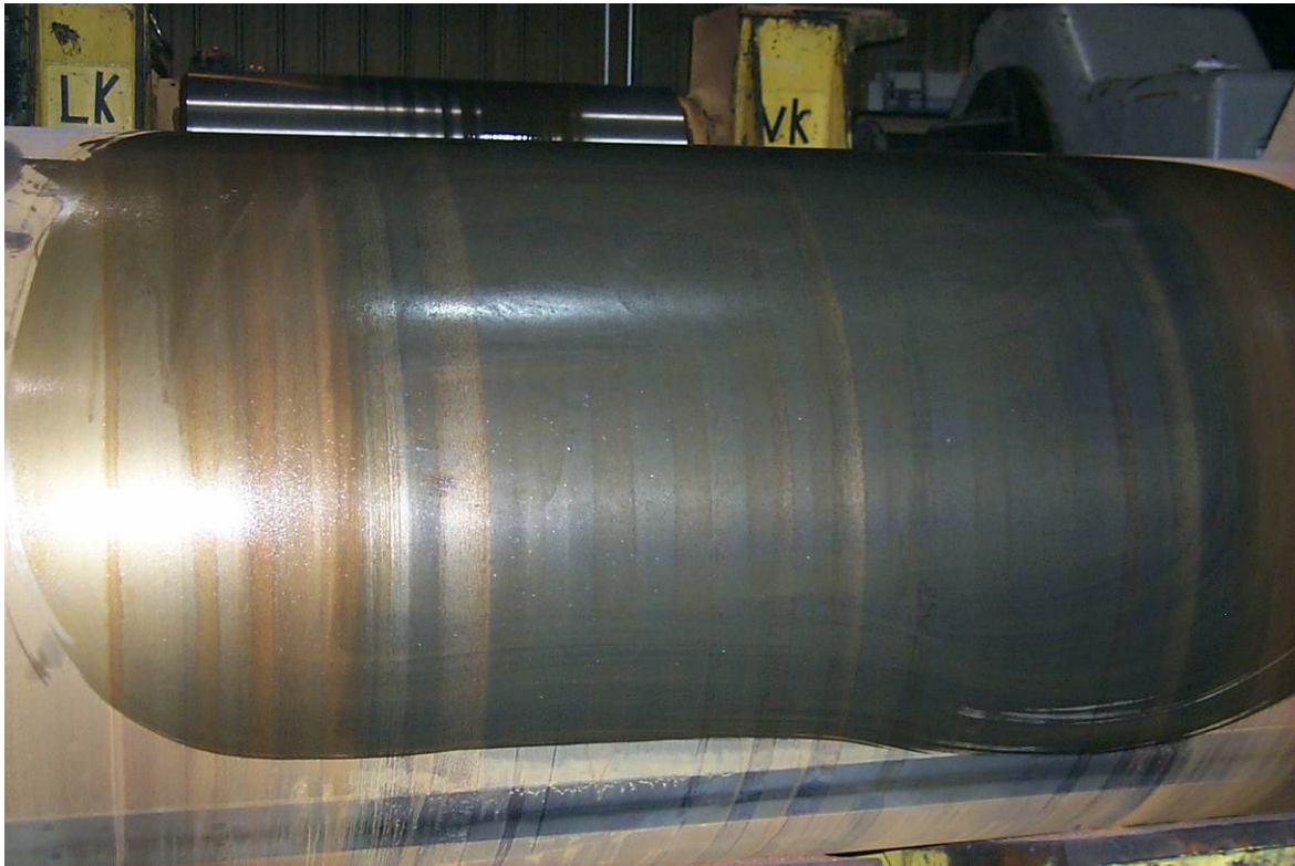
Figure 3: Semi-HSS roll in a European rolling mill after approx. 80,000 t.
