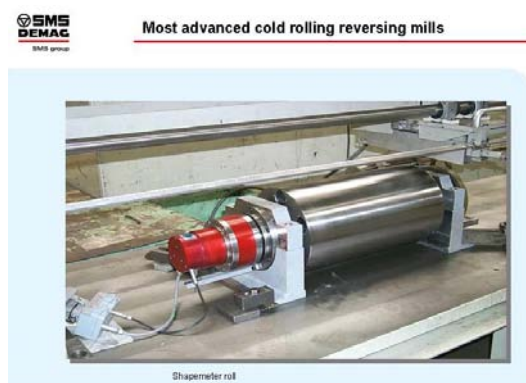
Figure 16. Solid shapemeter roll for optimized flatness control
