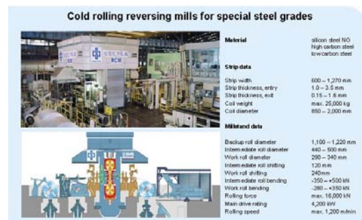
Figure 10. Cold rolling reversing mills for special steel grades
