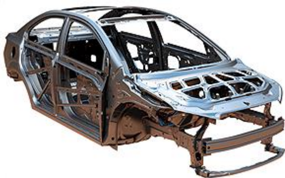
Figure 3: Decreasing the weight of the "Body in White" (BIW) Figure 4: BIW for European car manufacturers
