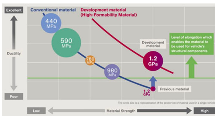
Figure 1: Properties of available steel grades
