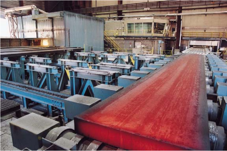
Figure 10. In line CASTTGRIND® plant for stainless steel slabs at Outokumpu, Tornio, Finland
