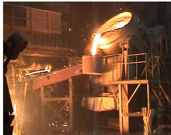
Figure 8 Feeding Hot Metal into a Consteel® EAF
