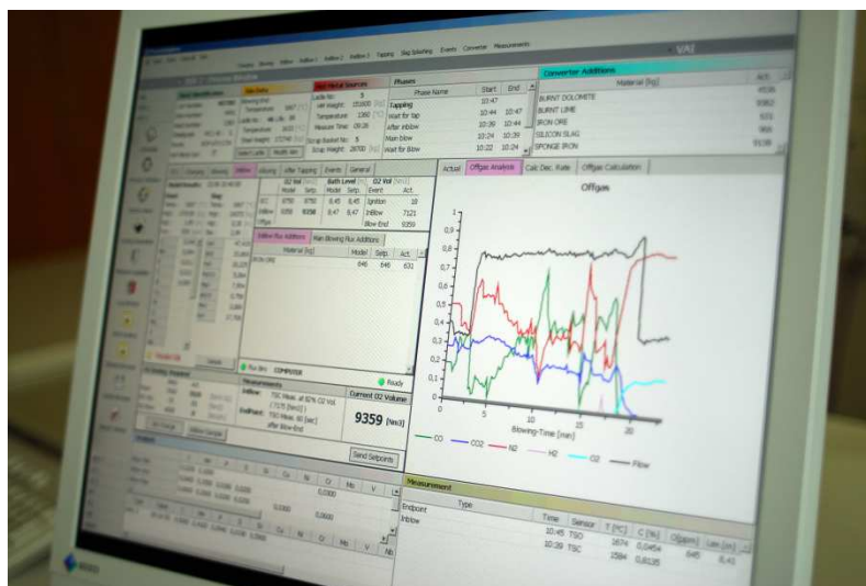
Figure 6: Graphical SIMETAL BOF Optimization visualization system.
