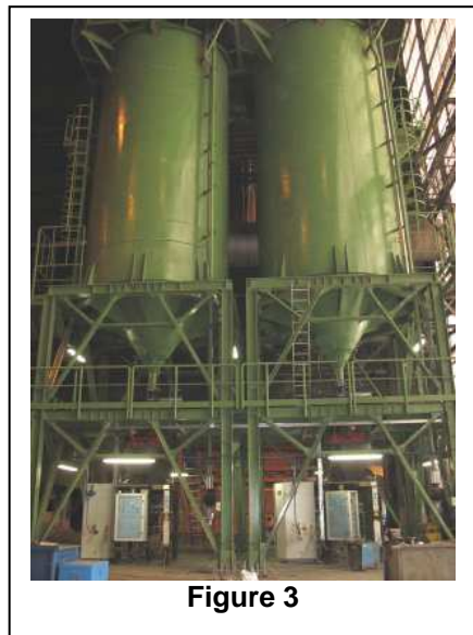
Figure 3 and 4: Two dedicated MOLI dispensers installed under two 125 m 3 storage silos
