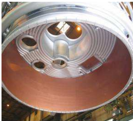
Figure 5. LMF copper roof.
