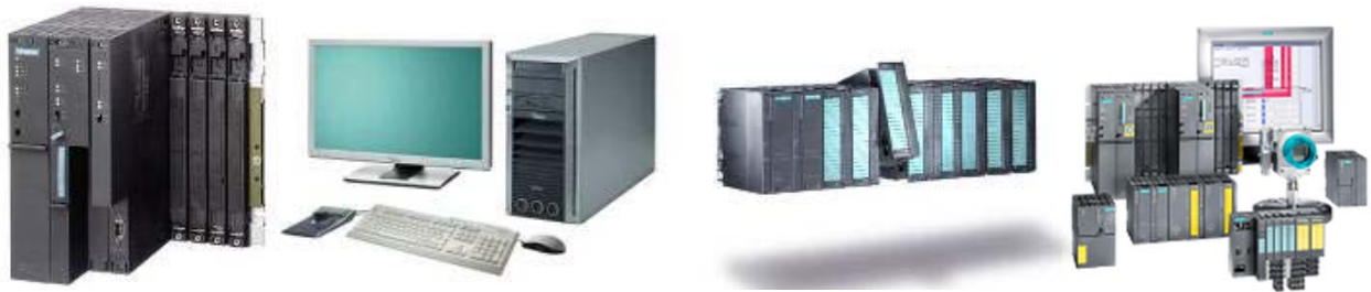
Figure 10. Hardware components of the Siroll automation system.
